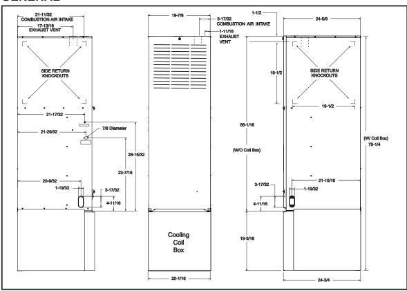
Figure 1. Furnace Dimensions
